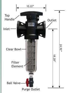
For flow levels up to 150 US gpm, the T2C-HF-200 is designed for rugged industrial uses. Perfect for heavy duty applications that require a easy to clean screen filter. Included ball valve ensures a leak-free purge.
